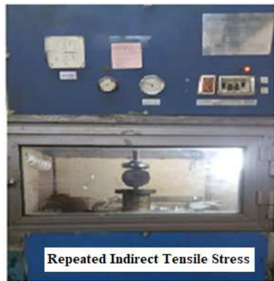
Figure 2. Repeated indirect tensile stress test in progress in the PRLS.
