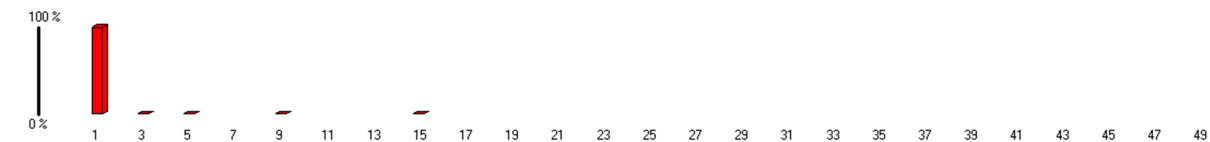
Figure 11. Occurrence of odd harmonics in the voltage without voltage unbalance.
