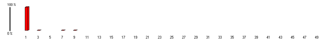
Figure 11. Occurrence of odd harmonics in the voltage without voltage unbalance.
