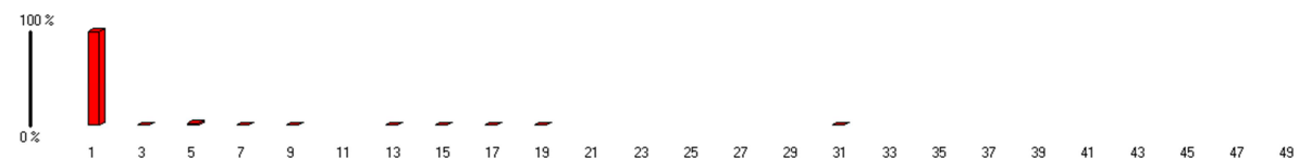
Figure 8. Harmonic components of the motor supply voltages with the undervoltage effect in Phase B.
