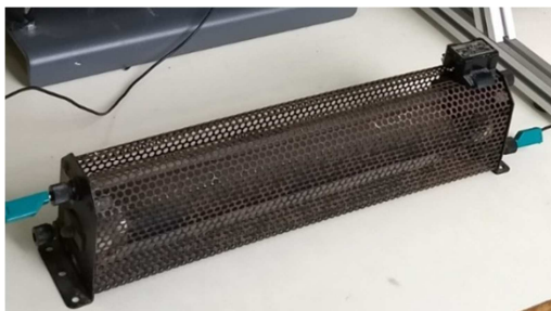
Figure 3. 103Ω and 545W Rheostat.
