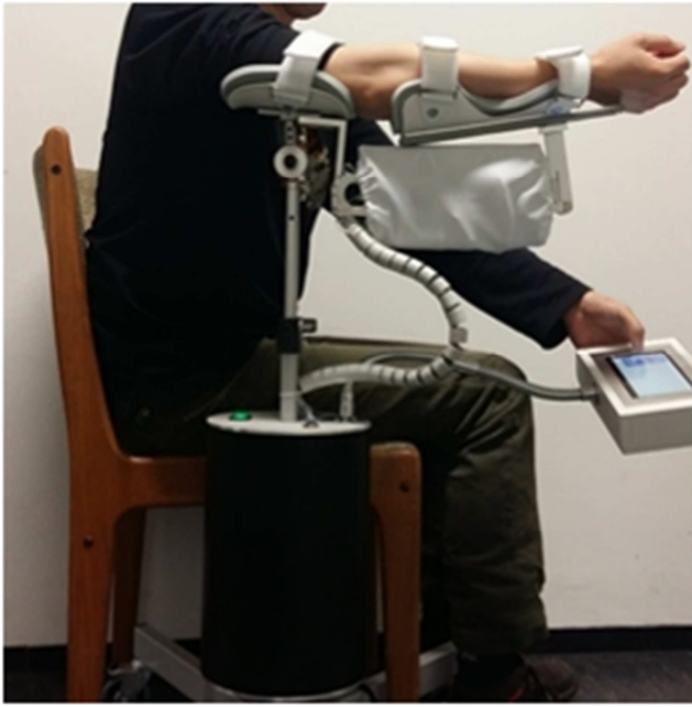
Figure 2. Pneumatic elbow trainer: Prototype of a compact elbow trainer with integrated compressed air supply and assistive control system based on position sensors only. A touchscreen as control interface is used to make controlling more convenient.
