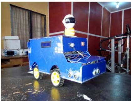
Figure 14. The fully designed, constructed and tested proposed autonomous vehicle with integrated sensor suite based on the IoT technologies for obstacle detection and avoidance, gas and smoke detection as well as wireless streaming video transmission of the real-time camera coverage to remote base location.
