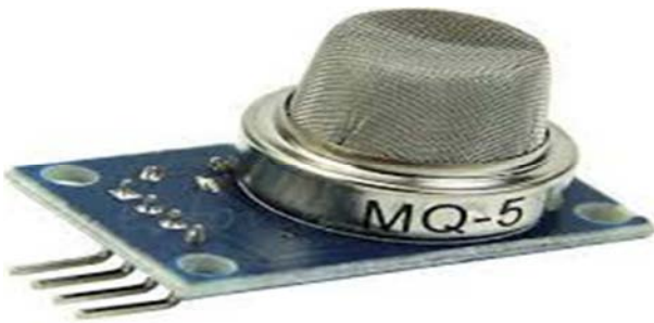
Figure 3. The MQ-5 sensor-based gas detector.
