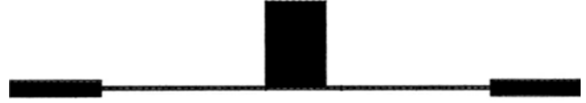
Figure 2. The conventional structure of the Low pass filter with open circuited stubs.
