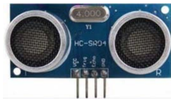
Figure 6. The HC-SR04 ultrasonic sensor.
