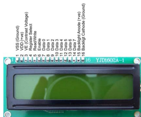
Figure 7. The physical picture and pin definition of the YJD1602A-1 16-by-2 LCD display module.
