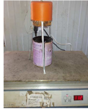
Fig. 2. Blending of modified asphalt cement.
