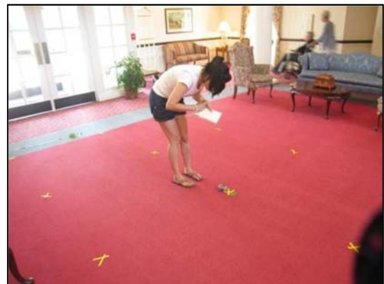
Figure 2. Researcher records light meter readings on the floor of the Lobby.
