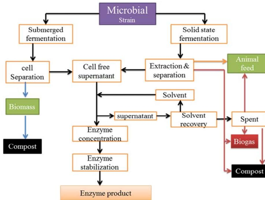
Figure 4. Process flow chart for clean enzyme production and purification.
