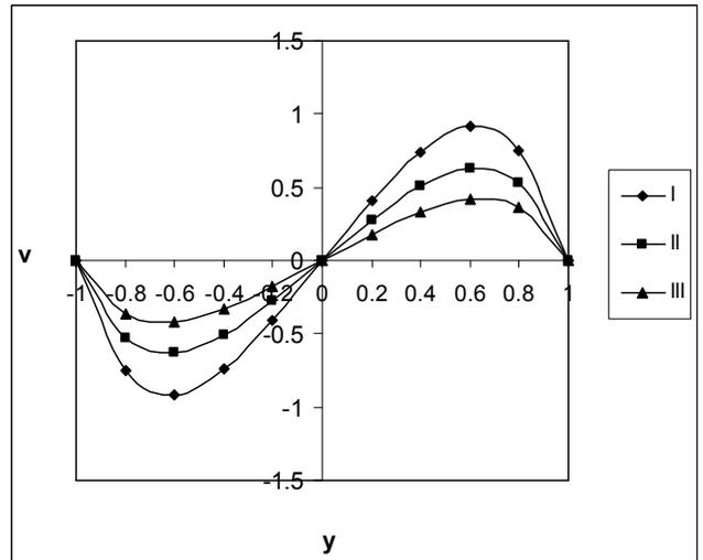
Figure 4(b). Secondary Velocity for various values of  $Q$ .
