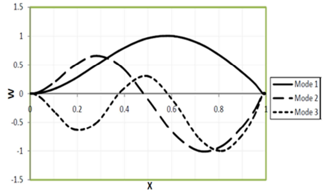
Figure 6c. The first three mode shapes of uniform Clamped-Simply bar ( K_f=1.0 ).
