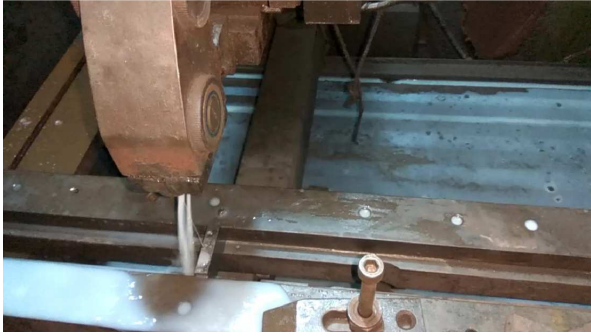
Figure 4 Overview of slot cutting operation by CNC wire cut machine.
