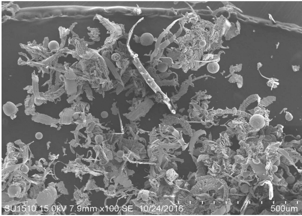
Figure 7. SEM micrographs of the chip at the down feed of 30 \mu m
