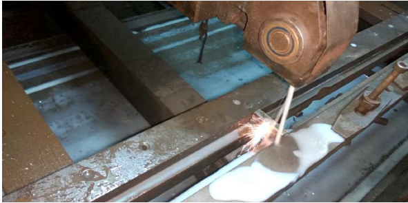
Figure 5 Overview of slot cutting operation by CNC wire cut machine.
