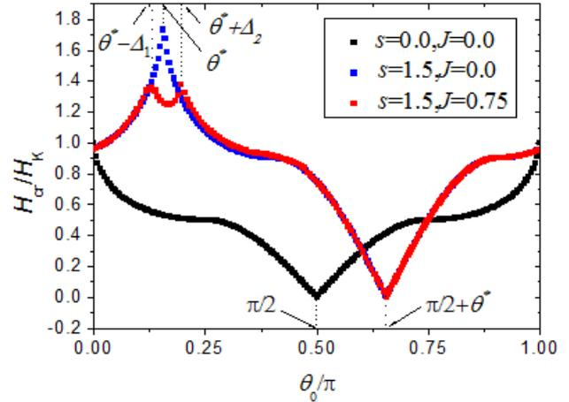
Figure 5. The angular dependence of the coercivity for  $s=0.0, J=0.0$ ,  $s=1.5, J=0.0$  and  $s=1.5, J=0.75$ . ( $s = H_\sigma / H_K$ ).
