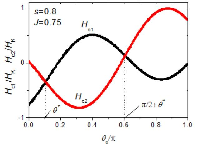
**Figure 3.** The angular dependence of  $H_{c1}$  and  $H_{c2}$  ( $s = H_\sigma / H_K$ ).
