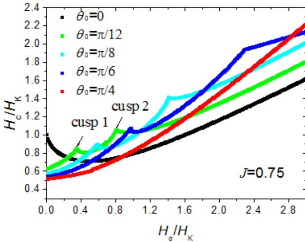
Figure 4. Coercivity curves as the function of stress intensity for an exchange bias system.
