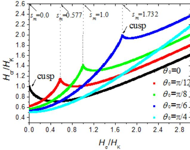
**Figure 2.** Coercive force changing as the function of stress intensity,  $s_m$  stands for the value of  $H_\sigma/H_K$  at the peak position.
