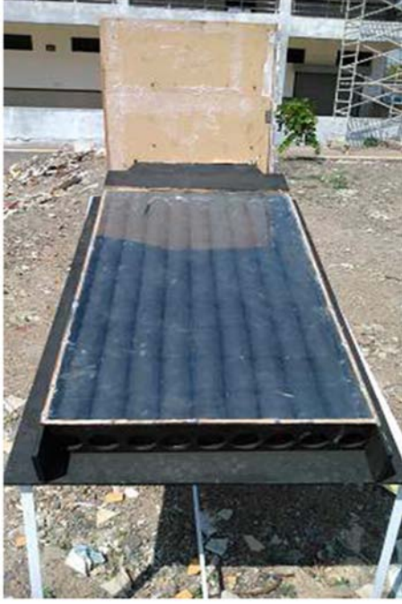
Figure 2. Photograph of experimental setup (Actual Indirect-Type Passive pop can solar dryer).
