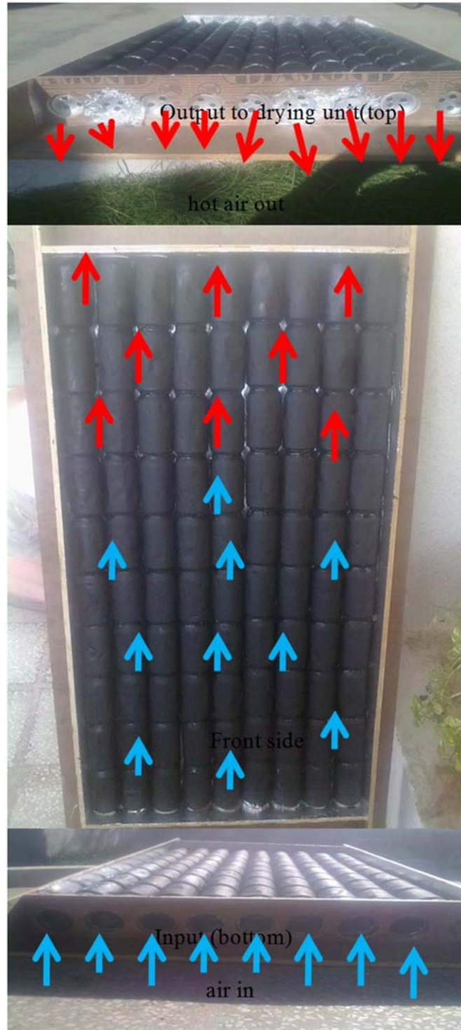
Figure 1. Working mechanism and schematic view of pop can collector.
