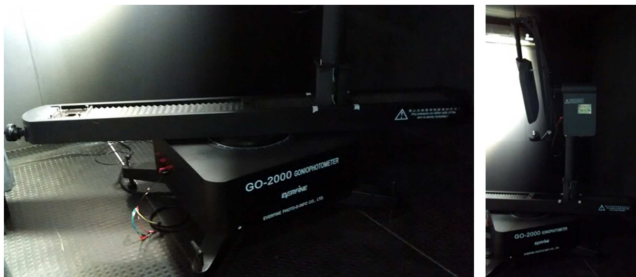
Figure 4. Test illustration of LED luminaire using the Gonio photometer.
