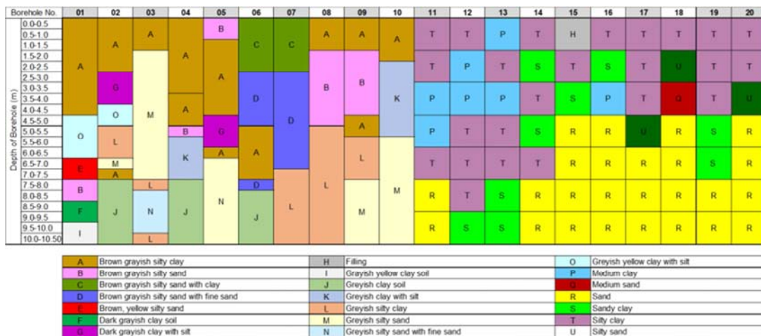
Figure 9. Borehole Log showing the Details of Soil Layers of Twenty Boreholes.
