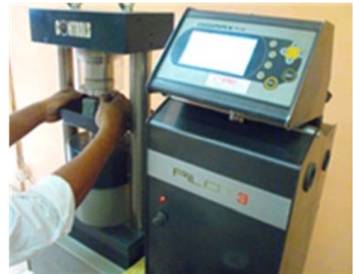
Figure 10. Measuring compressive strength.
