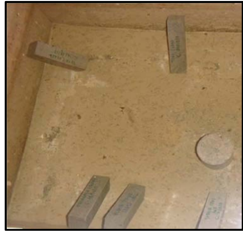
Figure 9. Conservation of test-tubes.
