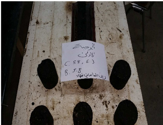
Figure 3. Part of the prepared cylindrical specimen for temperature susceptibility.
