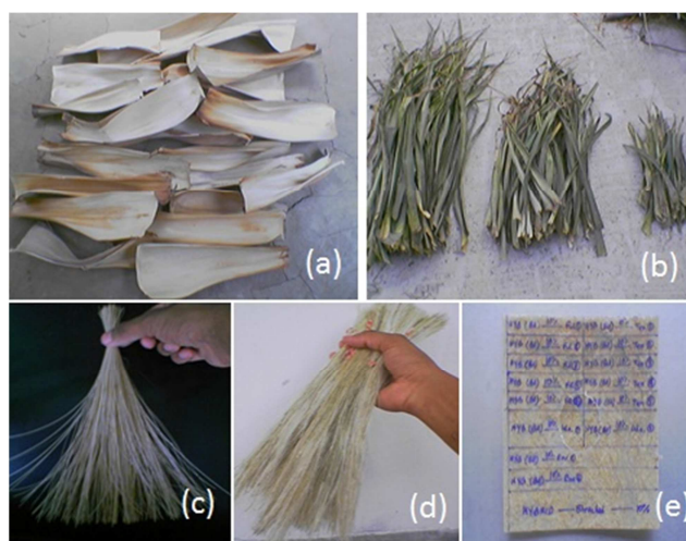
Figure 1. Image of (a) areca palm leaf, (b) pineapple leaf, (c) areca palm leaf fibers, (d) pineapple leaf fibers and (e) short hybrid fiber/PP composite.
