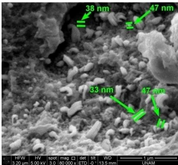
Fig. 7. SEM image of CNC prepared from cotton sonicated for 120 min and 40 % acid.
