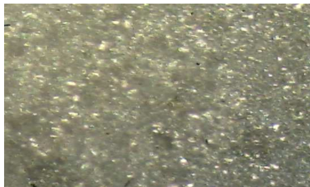
Figure 11. Specimen structure immersed in 5% H 2 SO 4 with pomegranate peel at X200.
