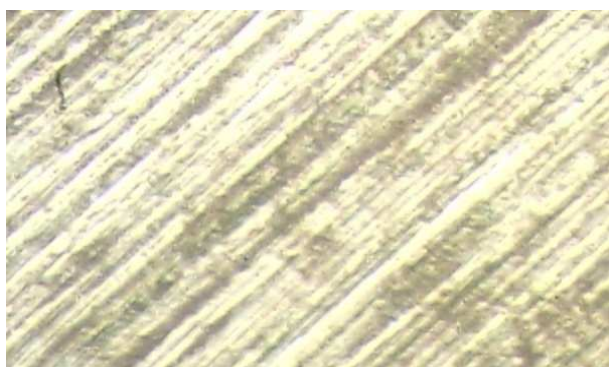
Figure 10. Specimen structure immersed in 5% H 2 SO 4 at X200.
