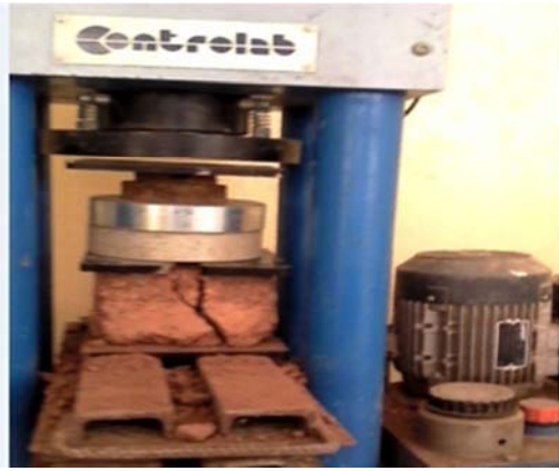
Figure 9. Testing of Compressed Lateritic Soil Blocks by Hydraulic concrete press.
