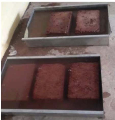
Figure 10. Capillary immersion and suction of the blocks.
