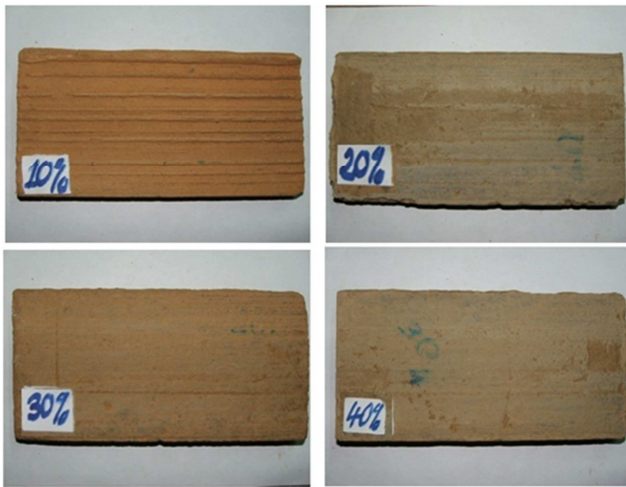
Figure 3. Surface condition of the blocks after wear.
