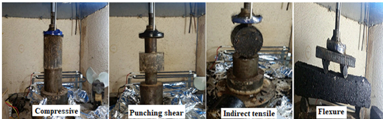
Figure 2. Testing technique of the prepared specimens.
