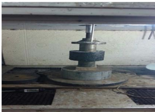
Fig. 3. Repeated double punching shear test.
