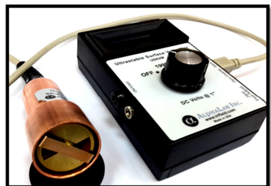
Fig. 3. Electrostatic field measuring device.
