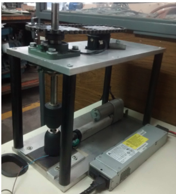
Figure 1. Fatigue testing machine for torsion and torsion-bending testing (in process of patent, 2015).
