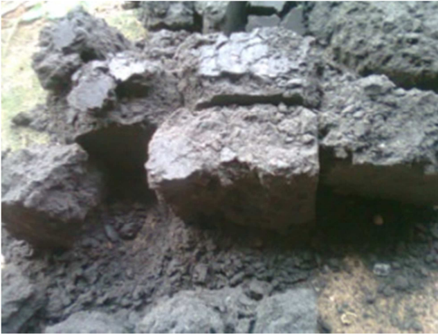
(b) 100% RHA specimen after testing for setting time.
