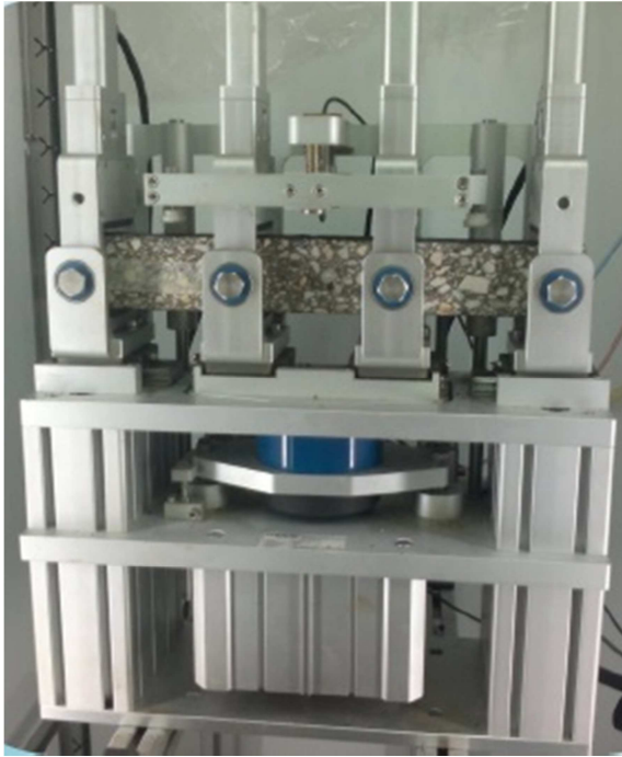
Fig. 6. Flexural Fatigue Test in process
