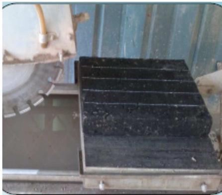
Fig. 2. Sawing beam specimens from slab
