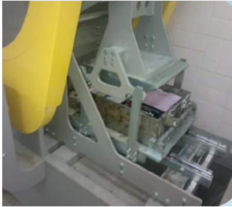
Fig. 1. Preparation of roller compacted slab
