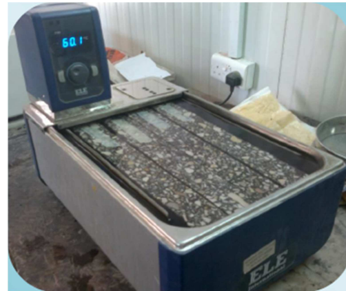
Fig. 4. Conditioning the beams in Water Bath
