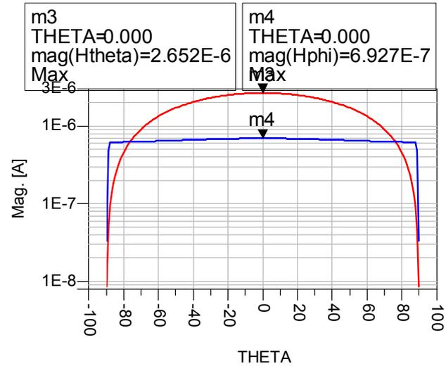
Figure 4. Simulated Radiation Pattern H(Q) for triangular patch (0.00035) and (35).
