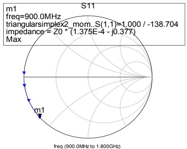
Figure 2. Simulated Input Impedance for triangular patch (0.00035) and (35).
