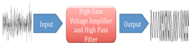
Figure 2. Receiver Block Diagram.
