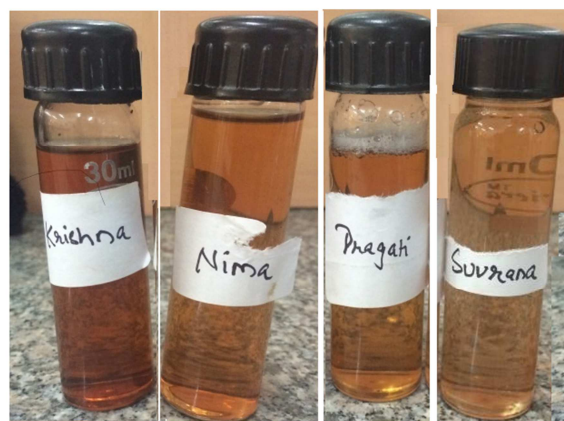
Figure 2. Photographs depicting synthesis of silver nanoparticles after 24 h of incubation of reaction mixture containing 1 mM silver nitrate and lemongrass extract (9:1 v/v).
